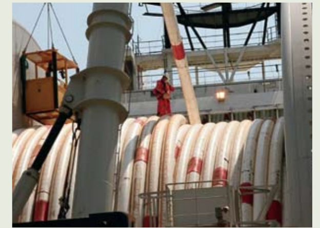
Subsea pipe spooled and ready
